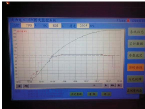
Fig. 8. Starting Speed and Y and \Delta Loop DC Side
